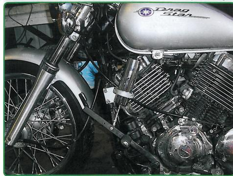
First disconnect the battery (if you Mig weld with the battery still connected it may damage the electrical system of the bike.
