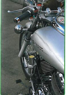
space between them and the handgrip. I did find that when using the indicator switch I was in danger of hitting one of the gear changer buttons. I solved this by moving the gear changer buttons round the handlebar a bit more, which in fact I found much better as my thumb is more under the grip of course than level with the indicator switch making it easier to change gear as the thumb didn't have to move so far.
